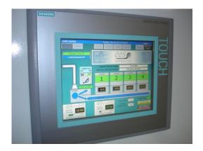
The *UltraLoft* UL/CE compliant system is designed around off the shelf components manufactured by Siemens, Allen Bradley and others. The *UltraLoft* PLC based touch screen control system includes features such as receipt management, equipment auto start/stop, active weight control, alarming, graphs, trending, spreadsheet reporting, help screens, remote online support and multilingual text.
