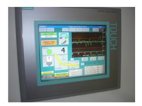
The new *UltraLoft* electronic weighing system is able to store hundred of blend receipts in the internal memory and on a typical flash drive. The *UltraLoft* system is actively correcting any variance in the fiber weight and/or percentage. The alarming feature will notify an operator if a hopper runs low of fiber. The *UltraLoft* system can be seen on the company's web site or demonstrated at your facility upon request.
